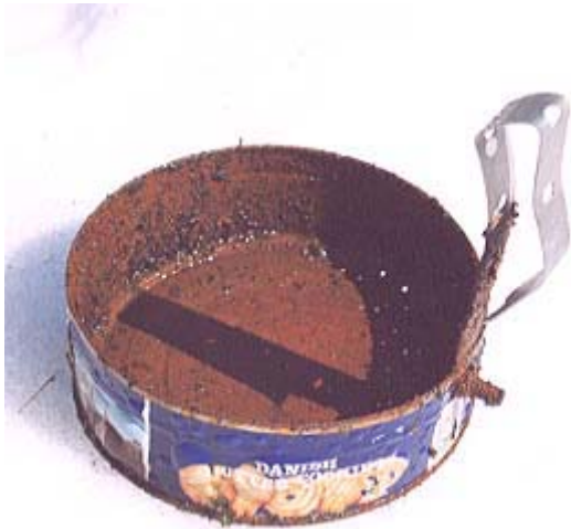
RIP! This is the sacrificial electrode. As you can see, the butter cookies are gone, as is the plating, parts of the label, and lots of metal.
